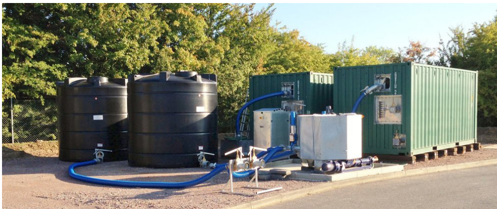
Figure 5 Modular digester used in the case study to process food waste, by Earthlee, n.d.
