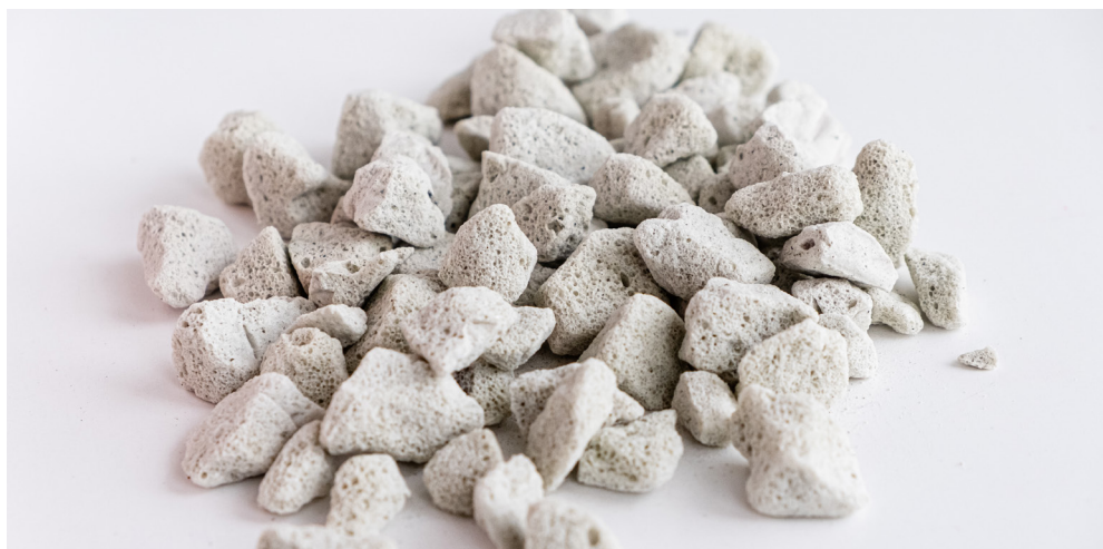
Figure 4 Foam glass aggregate has a wide variety of construction uses
