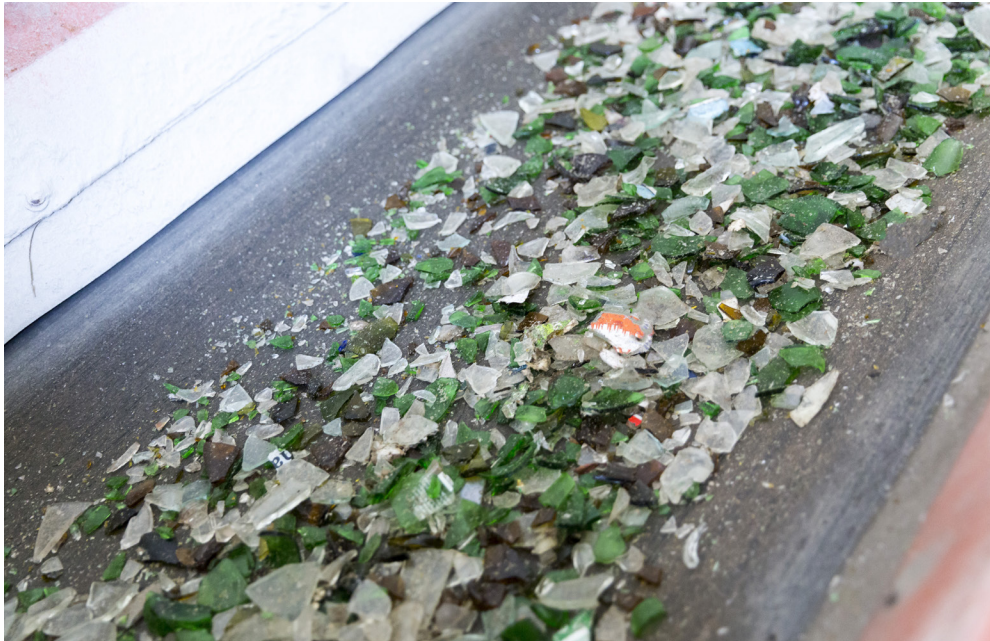
Figure 1 Small glass particles to be processed in a recycling facility
